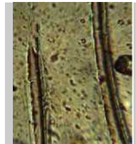
Photomicrograph showing where two fibers were pulled from an adhesive sampling tape leaving their colored coating behind. The coating is too thin to measure accurately with a standard microscope; however, it appears to be 180-600 nanometers, thinner than most bacteria.
